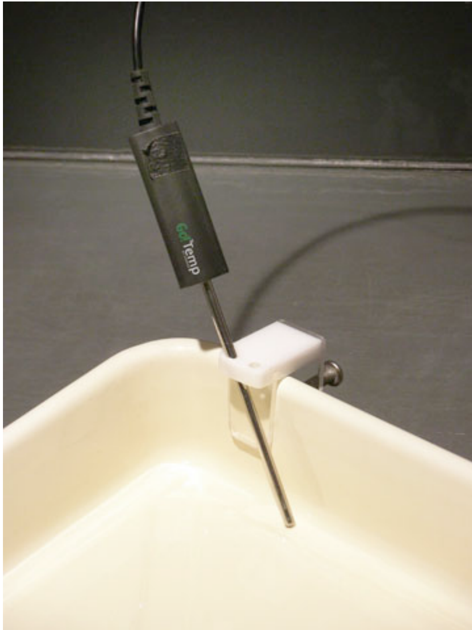
Figure A1-1. Ross clamp with Go!Temp probe attached to developing tray.
