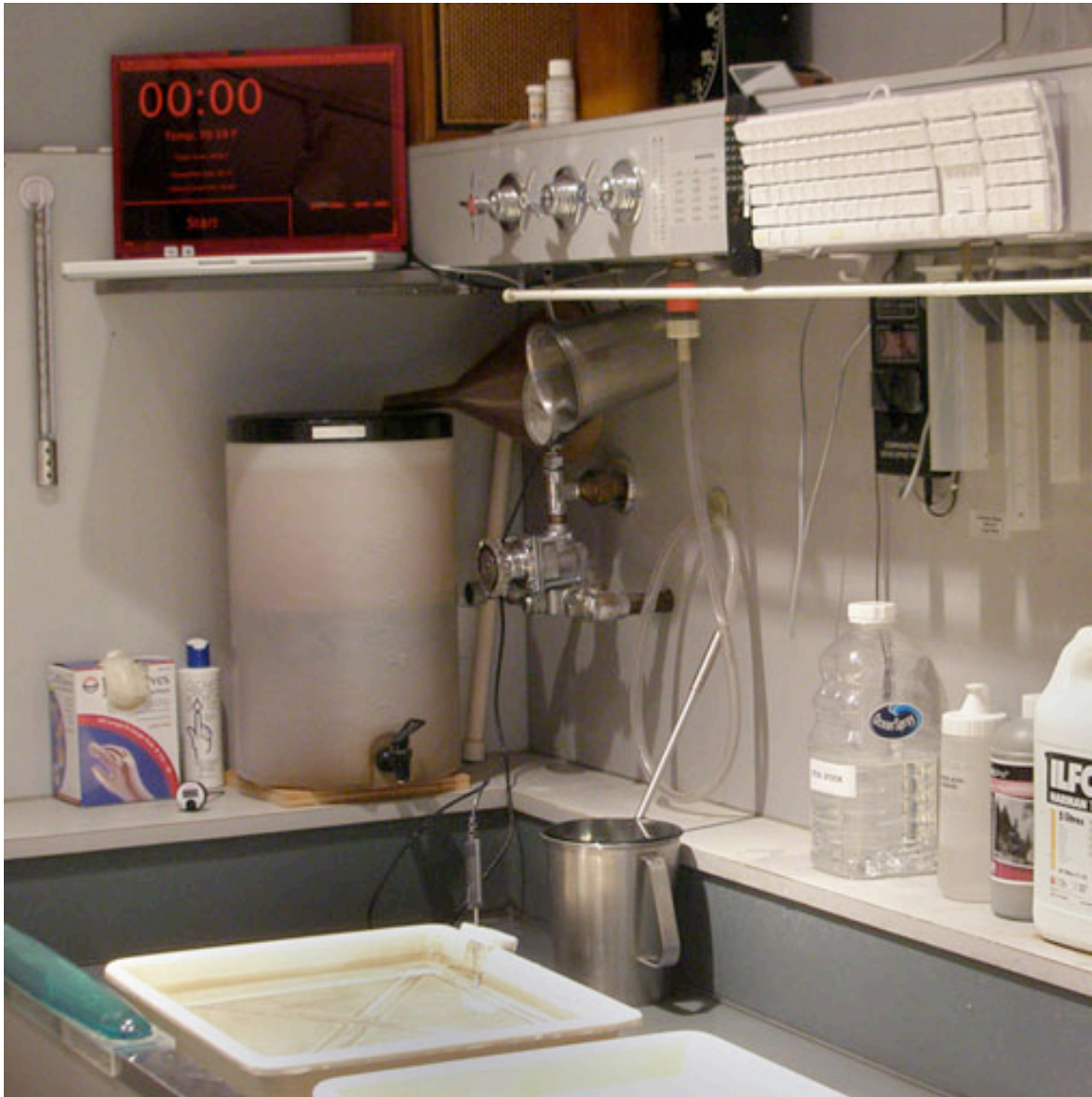
Figure 1. CompnTemp timer in Alan Ross's darkroom. The filter on the screen is a sheet of red acrylic plastic from the local plastic store. With this plastic filter in place, the monitor was tested safe against paper fog for at least 7 min exposure with the paper lying on the keyboard. Note the keyboard Alan has mounted over trays. It is connected to the laptop computer by its USB cable and used to control the timer. Any key, other than the number keys, can be used to start/stop the timer.
