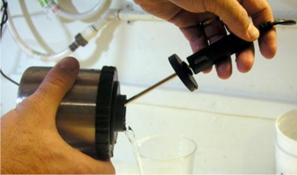
Figure A2-6 Emptying the tank with the temperature probe lid modification
