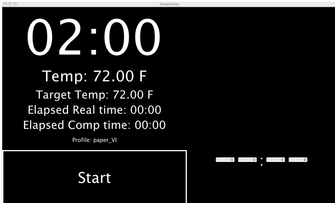
Figure 3. CompnTemp Main Window. The time is displayed at the top of the window. The current temperature, the target temperature and elapsed time and the real elapsed time are displayed below. A set of pull-down menus for setting the timer is on the right side of the window. The timer start time can also be set from the keyboard.
