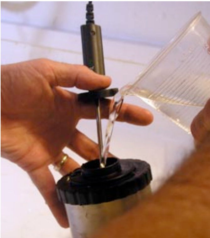
Figure A2-5. Filling the tank with the temperature probe lid modification
