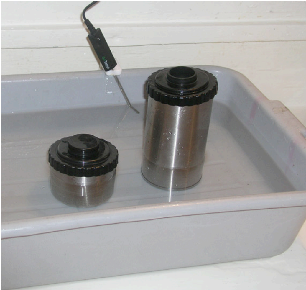
Figure A2-7. Tank Developing using water bath for temperature control
