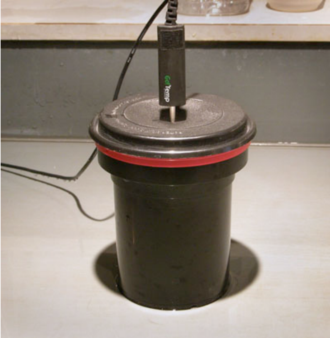
Figure 2. Go!Temp probe in Patterson tank. Tank was modified by drilling a small hole in lid. (thanks to Alan Ross for tank modification idea and photo).
